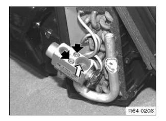
Unfasten screws and remove expansion valve.
